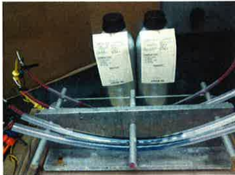
Fig. 1 TT5000 WTI and WTS detection time test setup.
